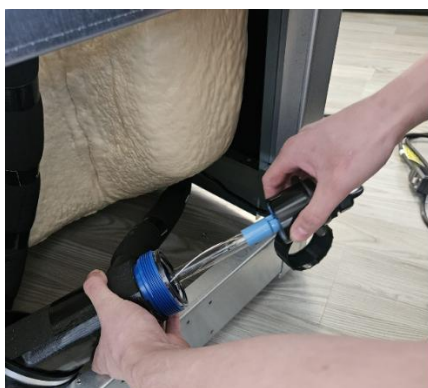
Fig. 12. Pull out/fit in UV-lamp
